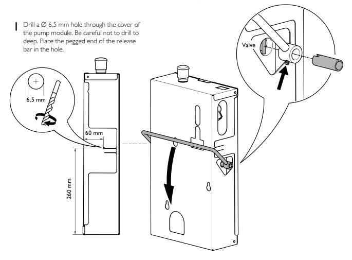
Ensure proper function by pushing down the release bar to open the valve and lower the platform.
