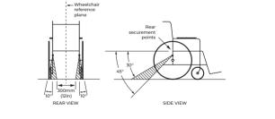
NOTE Note that angles indicated are obtained by projecting the angle of each tie-down strap onto a vertical plane parallel to the wheelchair reference plane (side view) or onto a vertical plane that is perpendicular to the wheelchair reference plane (rear view).
